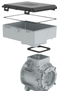
Figure 5 - Assembly of the terminal box
