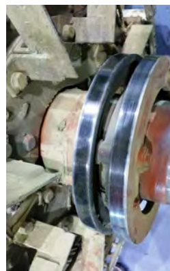
Contaminated collector ring treated with insulating varnish in the field
