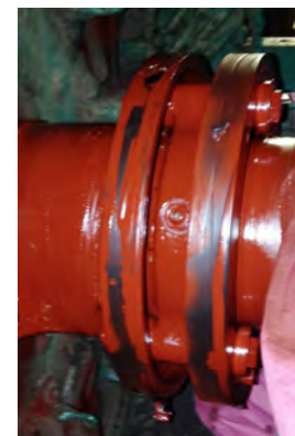
Contaminated collector ring treated with insulating varnish in the field
