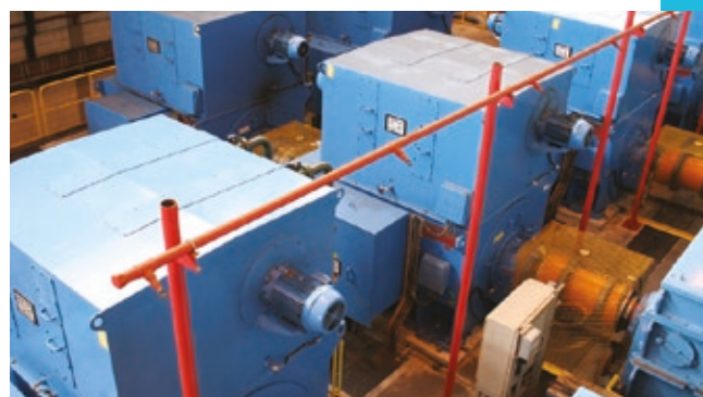
Synchronous motors SDL800, 3,000 kW, 3,100 V Application: rolling mills (iron and steel)
