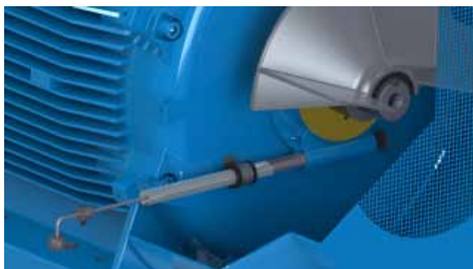
Figure 3.44 - Non drive end grease removal device
