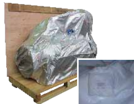
Figure 8.02 – Wooden seaworthy case - motor protection
