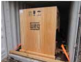
Figure 8.04 – Stuffing with lashing direct to motor eyebolts
