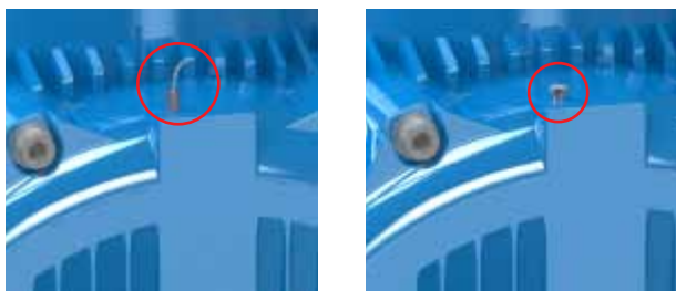
Figure 3.14 - Example of mounted vibration probes on W22Xd ribbed motors
