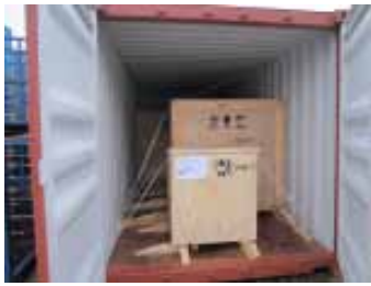
Figure 8.03 – Stuffing with lashing on the case
